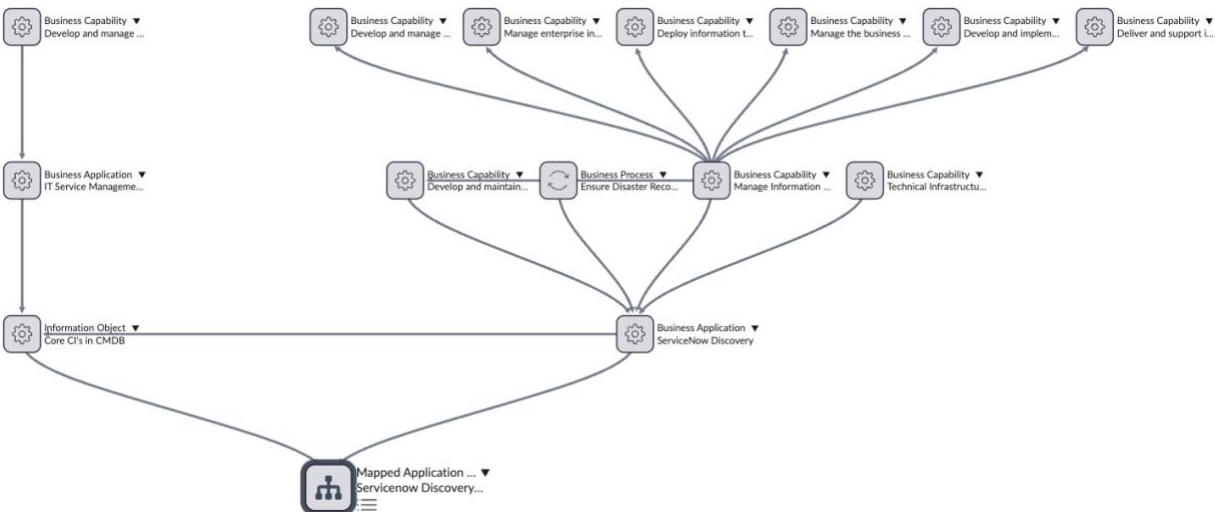
Figure 58 – Showing how the service instance “ServiceNow Discovery PROD” is related to both the parent business application “ServiceNow Discovery” and the Information Object (Type) “Core CIs in the CMDB”. We also see that the same Information Object (Type) has an upstream relationship to both “ServiceNow Discovery” and another business application called “IT Service Management”.
