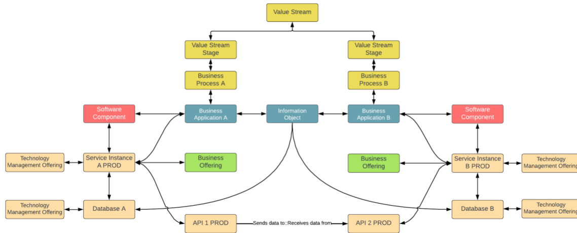
Figure 44 – Even without the Digital Integration Management feature in the Enterprise Architecture product it is possible to map out where data resides (at rest, red line) and where it is transmitted (API to API), as well as the business processes that use the information as part of a value stream.
